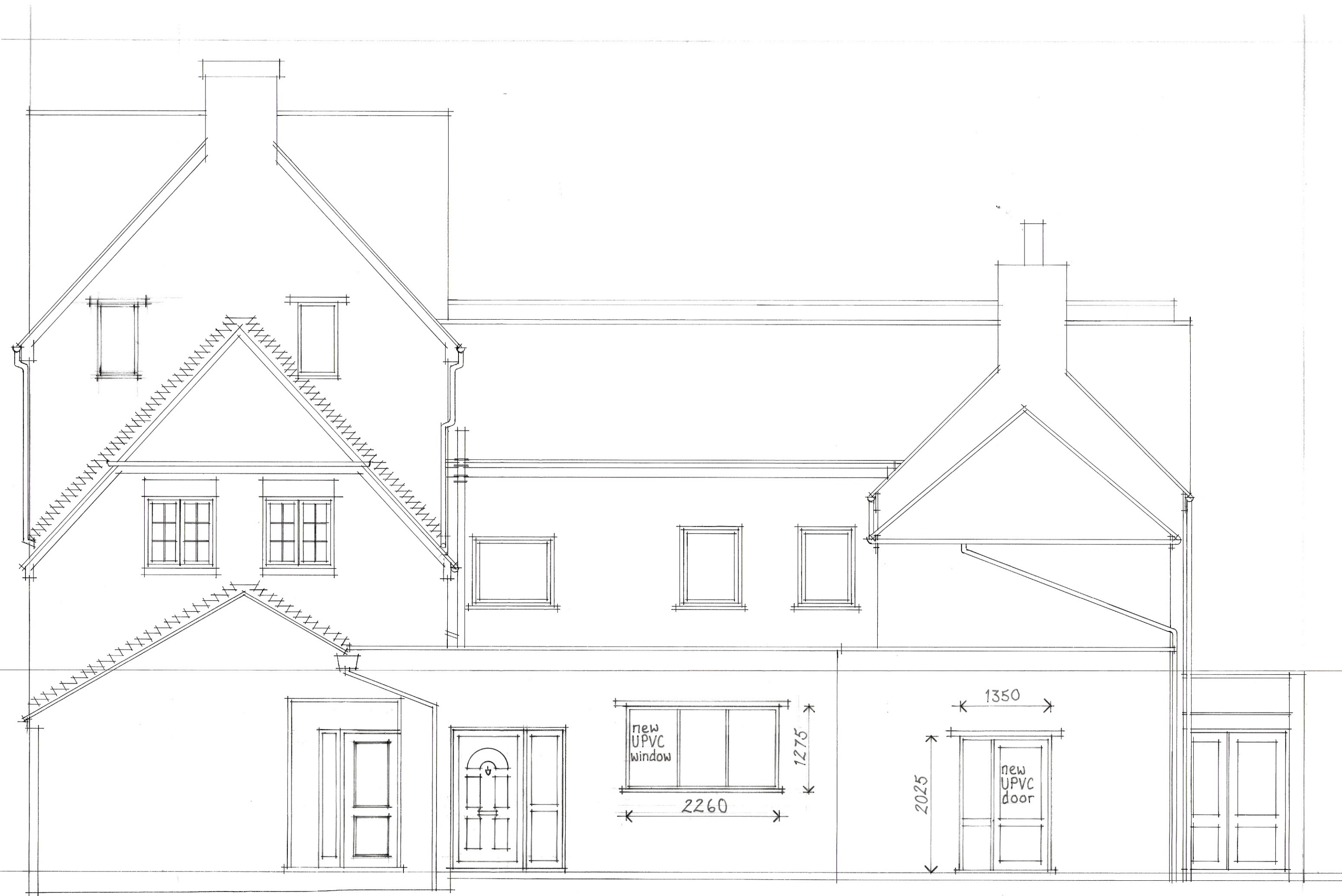
NORTH WEST ELEVATION AS PROPOSED
